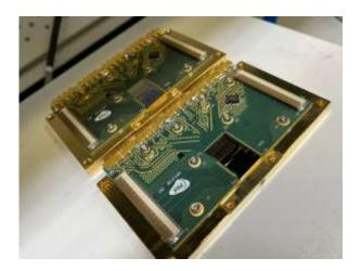
The evaluation board provides connectivity to all the integrated devices on the PIC. It allows customers to deliver 16 x 32Gbaud data lanes from coherent digital signal processors (cDSP) which map to 4 dual-polarization IQ modulated wavelengths.
